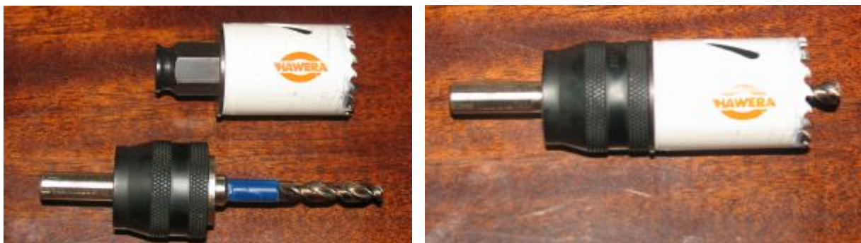
Fig. 4. Bi-metall bore HAWERA
